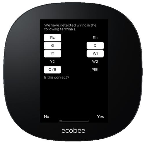
Ensure that Rc, G, Y<sub>1</sub>, O/B, C, and W<sub>1</sub> are the only wiring terminals highlighted then tap "Yes."
